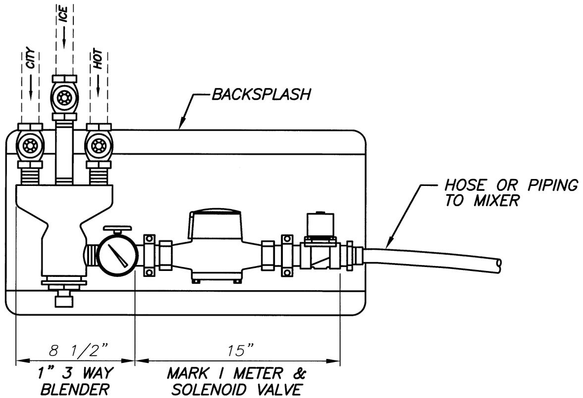
**FIG. 3 MARK I WITH 3-WAY MANUAL BLENDER**
