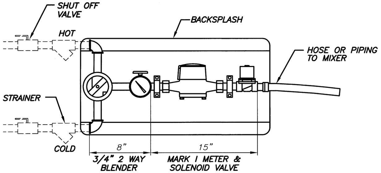
FIG. 2 MARK I METER & 2-WAY MANUAL BLENDER
