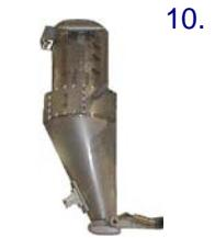
10. **Receiving hoppers** – Stainless or mild steel hoppers are generally mounted on electronic load cells to receive ingredients from the conveying system and discharge it into a mixer. The load cells are S-type stainless steel sealed units with precision bearing type suspension for superior performance. The load cells are carefully matched to the application for unsurpassed accuracy. The receiving hopper is equipped with a dust collector and vibratory and/or air fluidizer type discharge aids.
