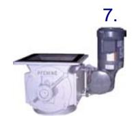
7. **Precision rotary airlocks** – For certain applications airlocks may be provided. Pfening has developed innovative rotor designs to improve airlock discharge accuracy. For this application, a variable frequency drive (VFD) is standard, allowing high-speed operation followed by a slow speed “dribble” for improved scaling accuracy. Cast iron, stainless steel and hard-chrome construction are available.
