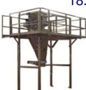
**18. Hopper support stands** – Pfening can provide support stands if it is impractical to hang the scale hoppers from the ceiling. These may be as simple as a four-legged structural framework or may include complex walkways, access/service platforms, and integral pipe and tubing supports. They may be for single or multiple hoppers. Stainless steel or mild steel construction is available.
