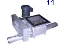
11. **Rotary feeder** – Precision machined, heavy-duty rotary vane, blow-through type feeders meter ingredients into either a pressure or vacuum conveying line. Standard construction is cast iron body with steel rotor. Includes rugged low-maintenance gearmotor with guard and chain drive. Stainless steel and hard chrome construction are also available.
