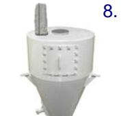
8. **Scale hoppers** – Stainless or mild steel hoppers are mounted on electronic load cells that weigh ingredients. The hoppers are sized for the application and generally have multiple inlet openings and an air filter. The load cells are S-type stainless steel sealed units suspended from vibration isolators for superior performance. The scale hopper is equipped with a butterfly valve discharge and has vibratory and/or air fluidizer type discharge.
