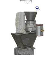
9. **Surge Hopper** – These isolate the scale hoppers from the conveying line. They receive the weighed ingredients and discharge them into a rotary feeder. An inlet butterfly valve provides complete isolation for the scale hopper from the disturbances of the conveying air, insuring maximum weighing accuracy. An air filter bag is provided to control dust and vent air in or out of the surge hopper. A level control is standard, along with vibratory or fluidizer type discharge.
