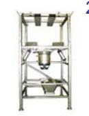
2. **Bulk bag unloaders** – For materials used in amounts justifying bulk bags of 1000 pounds or more, Pfening offers unloaders which feature integral hoists, spout connectors, paddle and/or vibratory dischargers, and feeders for connection to pressure or vacuum conveying systems. Bulk bags are set in place, the discharge spout is connected, and then it is automatically emptied by the discharger.
