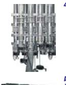
4. **Remote bin fill tubes** – Fill lines to each ingredient bin are manifolded into a hose connection station. Each tube is clearly marked and interlocked with limit switches to ensure that the proper material is loaded into each bin. The operator connects the hose from the bag dump or bulk bag unloader to the appropriate fill tube where the interlock controls confirm the material on the control panel.
