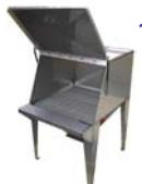
1. **Bag-dump stations** – Pfening bag dump stations are integrated into the pneumatic conveying system for remote filling of ingredient bins from bags or containers. These stations include a fully enclosed, stainless steel dump hopper, with safety grate and gas-spring assisted door. The dust collector may be integral or remote. A rotary feeder is mounted to the bottom of the unit.
