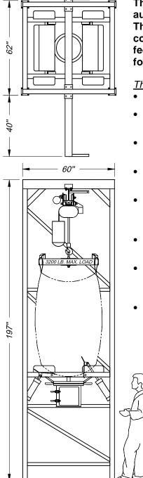
The Pfening Bulk Bag Unloader automatically discharges bulk bags. The material may be fed into an air conveying system or a mechanical feeder. A hoist and trolley is provided for lifting the bags into position.
